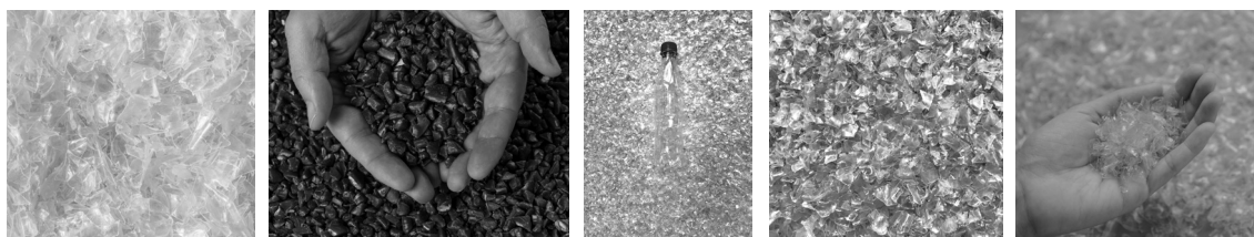
Figure 4.3: Variations in Polymer Translucency and Color from Virgin to Post-Consumer Recycled Plastic
